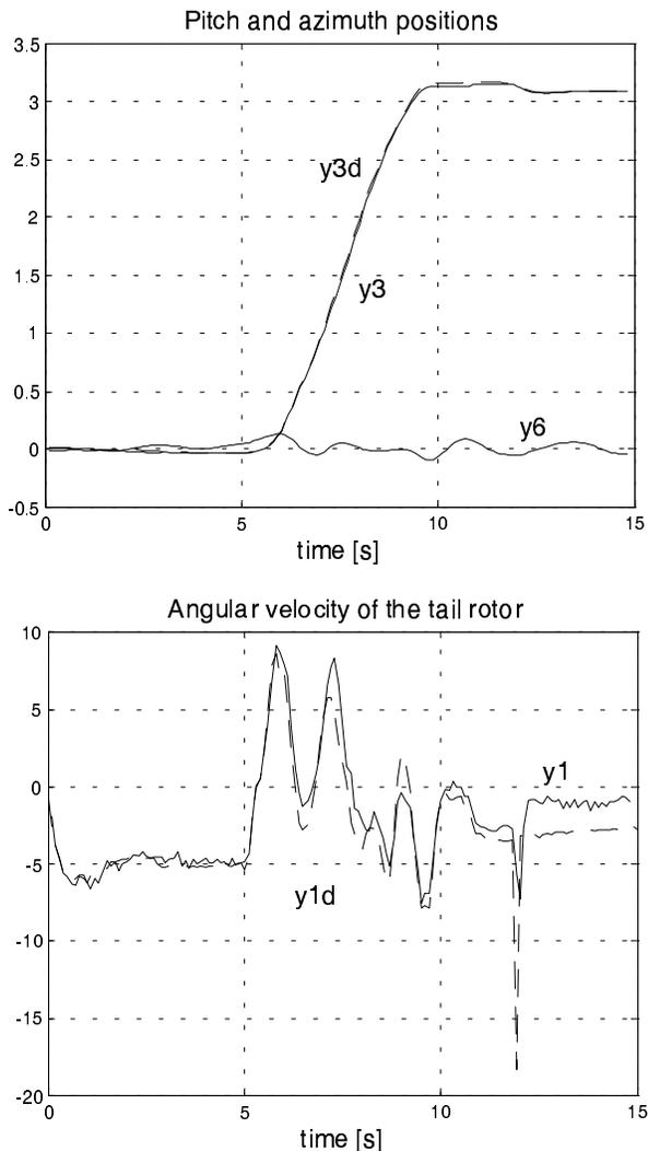
Fig. 10. Variable gain control. The dashed line represents the reference trajectory.
