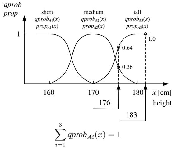
Fig. 7. Examples of the distribution functions  $qprob_{A_i}(x)$  of the qualification probability of the height  $x$  in the sets *short*, *medium* and *tall*. In this case the qualification functions are numerically equal to the property functions  $prop_{A_i}(x)$  of particular sets.
