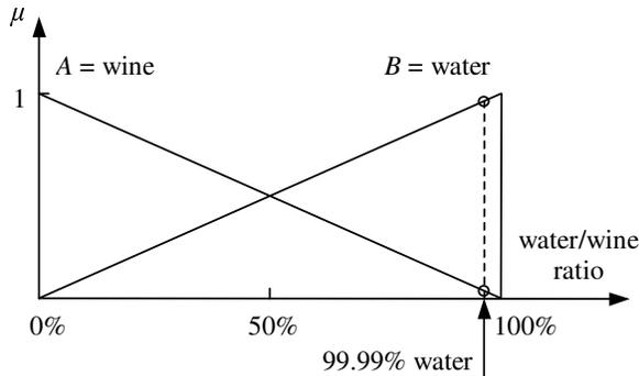
Fig. 1. Membership functions of the fuzzy sets  $A = \text{water}$  and  $B = \text{wine}$  characterizing the mixture of water and wine.
