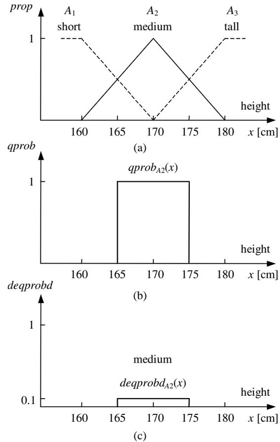
Fig. 5. Property functions  $prop_{A_1}(x)$ ,  $prop_{A_2}(x)$ ,  $prop_{A_3}(x)$  of height evaluations *short*, *medium*, *tall* (a), the distribution of the qualification probability  $qprob_{A_2}(x)$  of the elements  $x$  in the set  $A_2 = \textit{medium}$  height (b), and the distribution of the dequalification probability density  $deqprobd_{A_2}(x)$  that the element qualified in the set  $A_2 = \textit{medium}$  has the value  $x$  (c).
