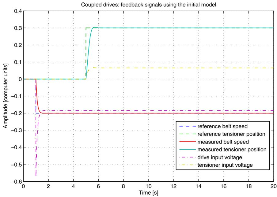
Fig. 3. Initial model verification.
