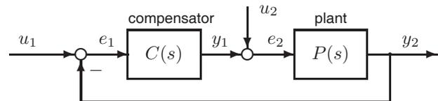
Fig. 1. Unity feedback system  $S(P, C)$ .
