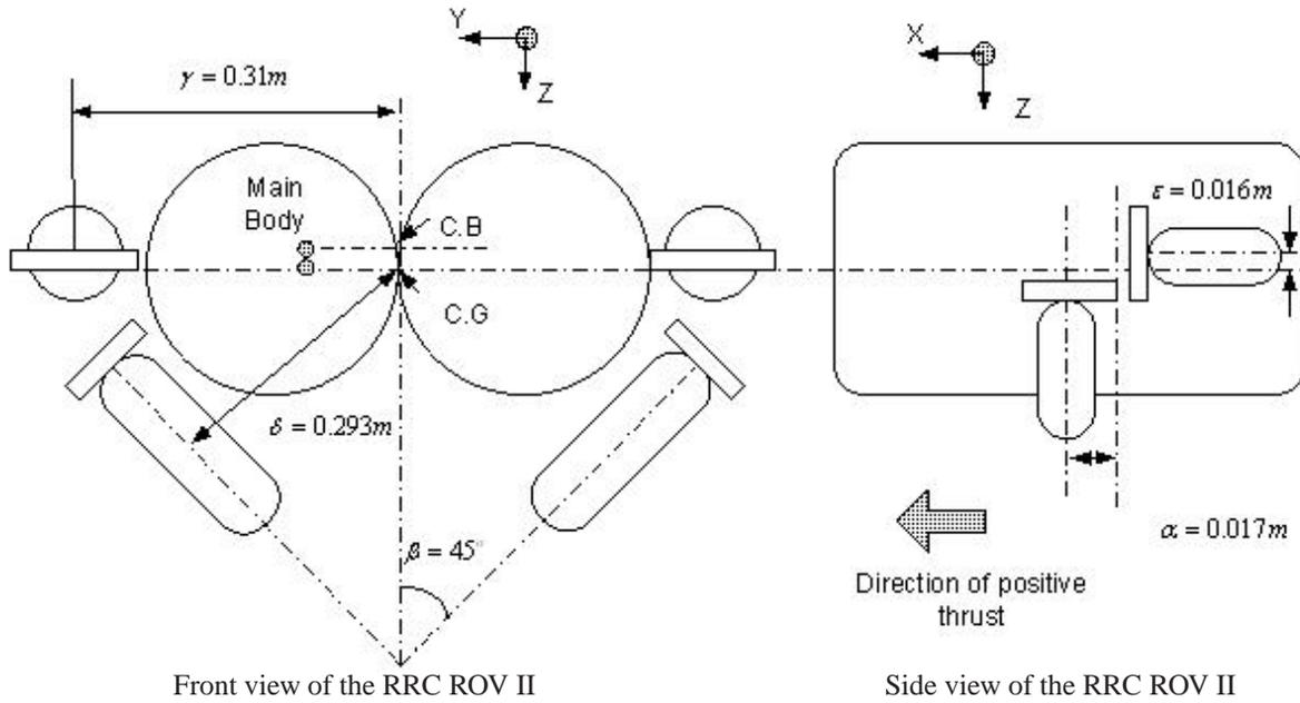
Fig. 1. Thruster configuration on the ROV platform.
