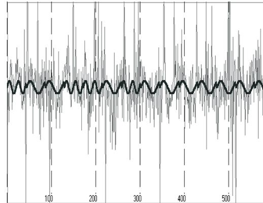
Fig. 3. Segment of the FSK signal with amplitude  $A_s = 10$  mV corrupted by a mixture of AWGN with variance  $\sigma^2 = 1000$  mV and impulsive noise with spike amplitude  $A_p = 200$  mV and the probability of negative and positive pulses equal to  $p = 5\%$ .
