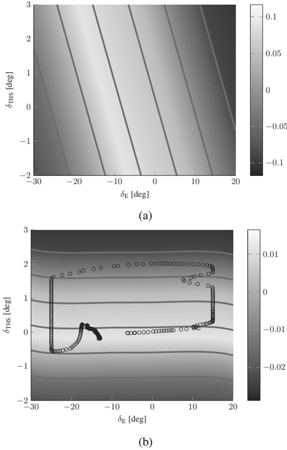
Fig. 7. Prior (a) and posterior (b) mean function of the GP modelling  $f_1(\mathbf{x}, \mathbf{u})$  in the 'stuck elevators' fault case. The surface is a projection of the mean function into the elevator-THS plane. The solid lines are contours of the surface. Circles indicate the location of the data accumulated.
