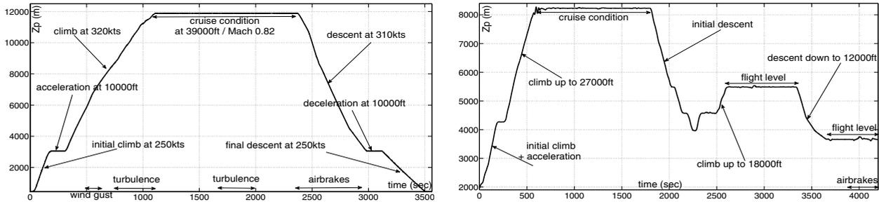
Fig. 7. Simulated (left) and real (right) flight profiles.
