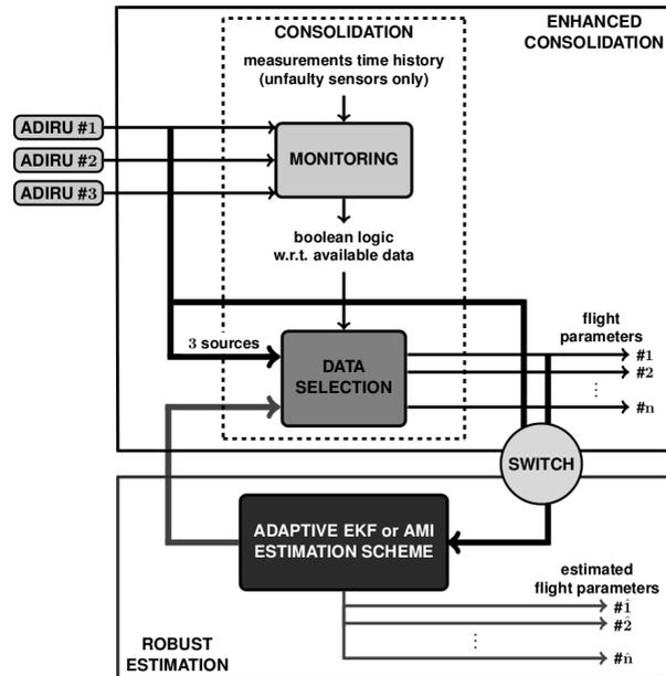
Fig. 1. Consolidation scheme using a virtual probe.
