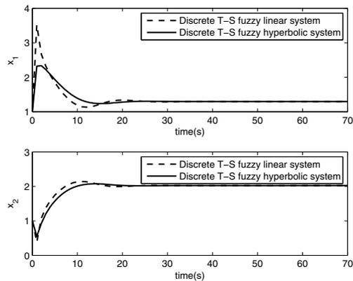
Fig. 2. State response curves and comparisons under the initial condition  $x(0) = [1 \ 0.55]$ . (DTSFSL: T-S fuzzy linear system, DTSFHS: T-S fuzzy hyperbolic system).
