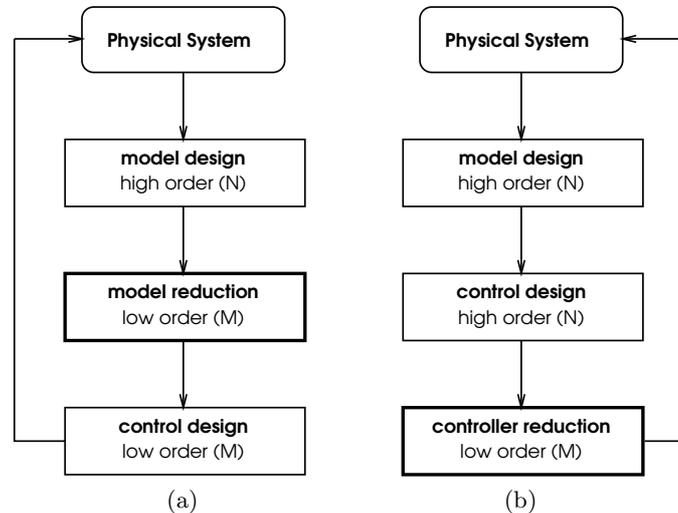
Fig. 1. (a) Reduce-then-design method, (b) design-then-reduce method.
