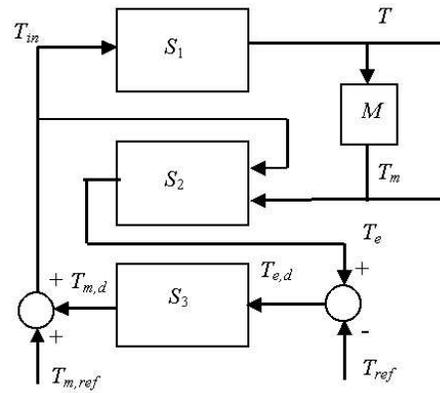
Fig. 6. Signal flowchart of the closed loop system.
