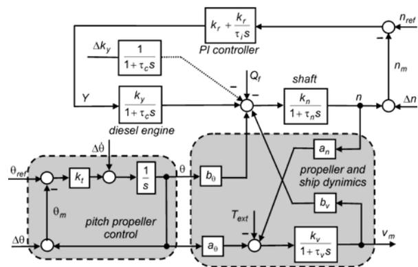
Fig. 12. Linearized model of the ship propulsion system.
