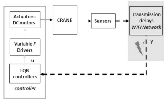
Fig. 3. Networked control overhead travelling crane scheme.
