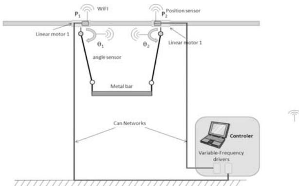
Fig. 2. Synoptic of the overhead travelling crane benchmark.
