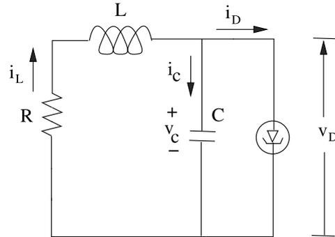
Fig. 1. Tunnel diode circuit (Assawinchaichote and Nguang, 2006).
