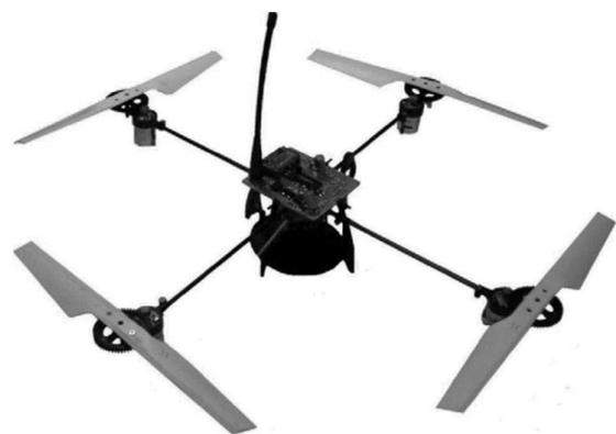
Fig. 1. Quadrotor mini-helicopter.
