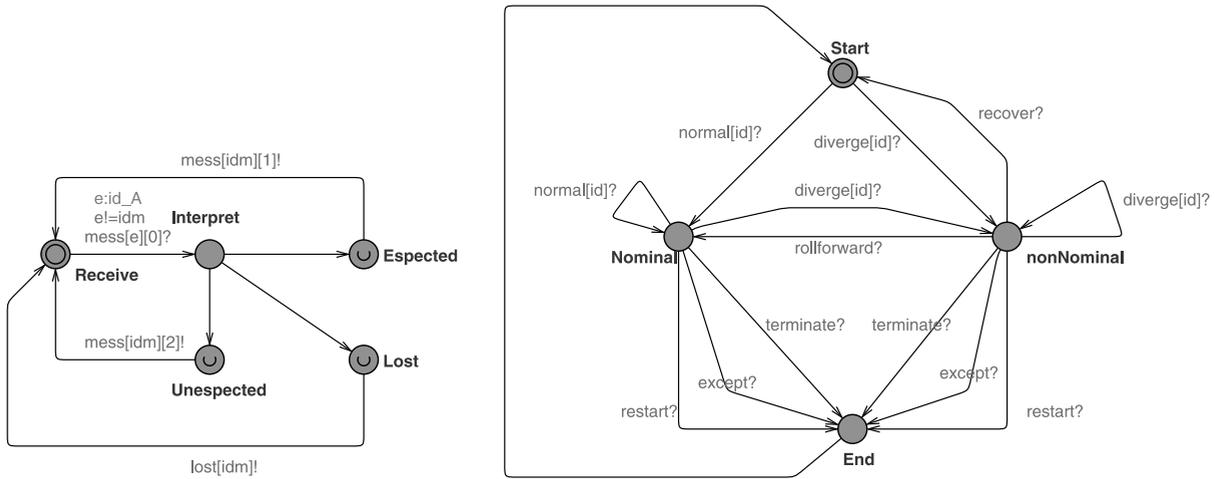
Fig. 7. ActorMessenger (left) and ActorInternalStates automata (right).
