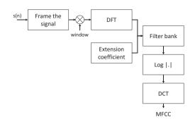
Fig. 1. Modified MFCC extraction process.
