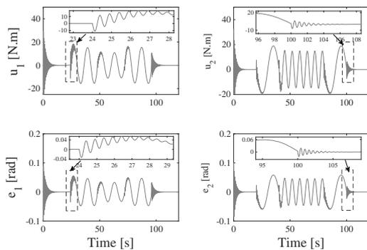
Fig. 6. Output tracking error and the control signal without external disturbances.
