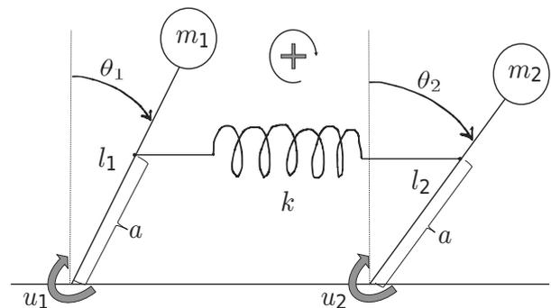
Fig. 4. Inverted pendulums connected by a spring.
