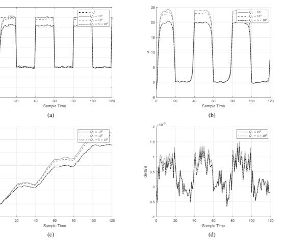
Fig. 4. System performance and degradation for different values of  $Q_1$ : system output (a), control input of the system (b), the degradation (c) and the rate of the evolution of the degradation (d).
