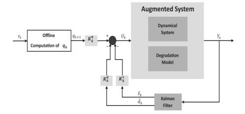
Fig. 1. Regulator design using state feedback and the Kalman filter as the observer.
