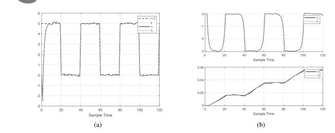
Fig. 2. Trajectory of estimated and real states and degradation in closed loop:  $x_{1,k}$ ,  $\hat{x}_{1,k}$  and the measurement  $y_k$  (a), the second state  $x_{2,k}$ ,  $\hat{x}_{2,k}$  and the degradation  $d_k$  and  $\hat{d}_k$  (b).
