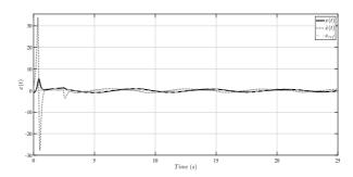
Fig. 5. Trajectories of the controlled system, reaching the reference  $x_{\rm ref}(t)=\sin 5t.$
