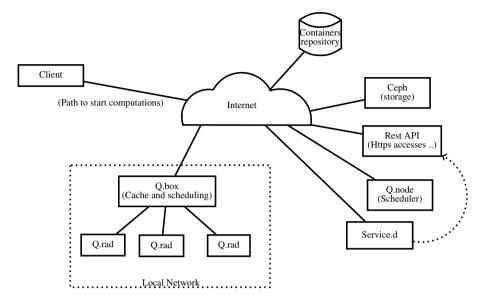
Fig. 1. Main components in the processing of a requests by Q.ware.
