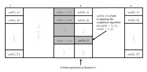
Fig. 7. Dynamic programming. The element sol(h, t) is generated at iteration h of the algorithm. Its computation is based on the first t elements of the column h-1.
