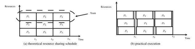
Fig. 4. Example of resource sharing schedules with three 9 parallel solvers.
