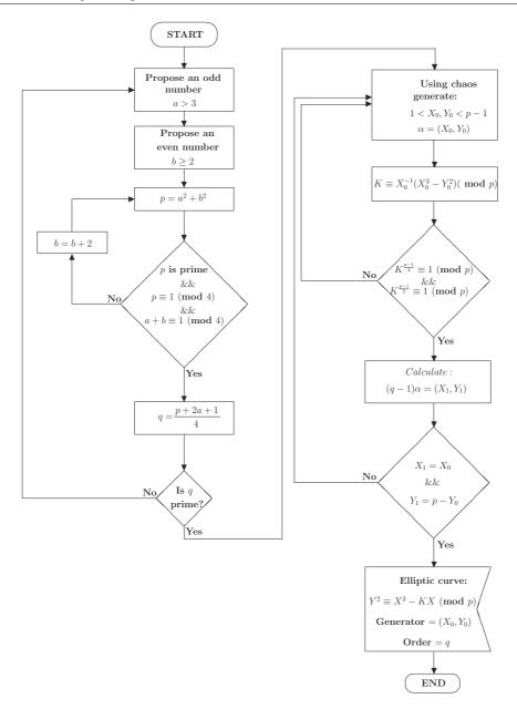
Fig. 1. Elliptic curve flowchart.
