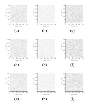
Fig. 3. Points (x<sub>c,d</sub>, y<sub>c,d</sub>) for the horizontal direction for the red (a), green (b) and blue (c) colors, for vertical direction (d), (e) and (f), and diagonal direction (g), (h) and (i), using the Lena test image encrypted with the *l* value.
