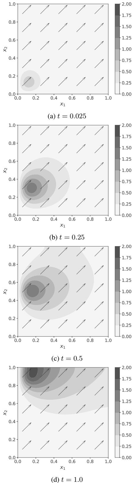
Fig. 2. Isolines of the contaminant concentration at consecutive time instants for a source moving in uniform motion from point  $(0.1, 0.1)$  to point  $(0.1, 0.9)$ . The arrows reflect the wind direction.
