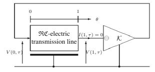
Fig. 4. Proportional feedback control of an  $\mathfrak{RC}$  transmission line.
