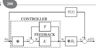
Fig. 2. Operator-theoretic diagram of the Lur'e control system.
