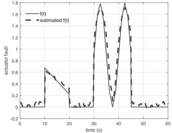
Fig. 2. Actuator fault  $f(t)$  and its estimate  $\hat{f}(t)$ .
