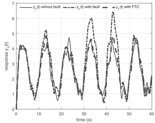
Fig. 3. Comparison of output  $y_1(t)$  in the following cases: without a fault, with a fault without FTC, with a fault with FTC.
