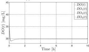
Fig. 12. Trajectories of DO(t) and its estimates  $\hat{DO}(t)$  for measurement S(t).
