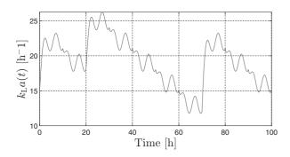
Fig. 4. Trajectory of gas-liquid transfer function  $k_{\rm L}a(t)$ .
