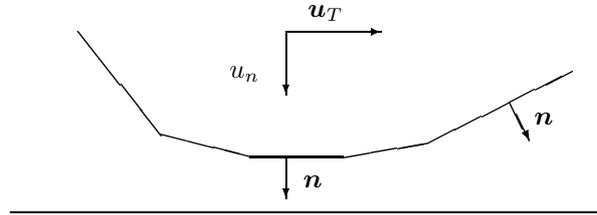
Fig. 4. Normal and tangential components.
