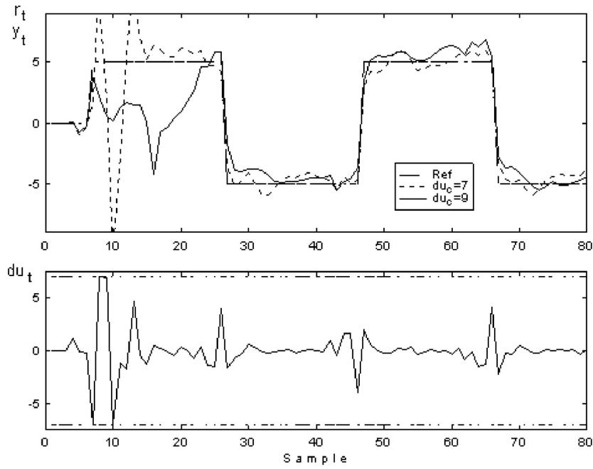
Fig. 5. STGPC under rate constraints (Example 3, ARIMAX).
