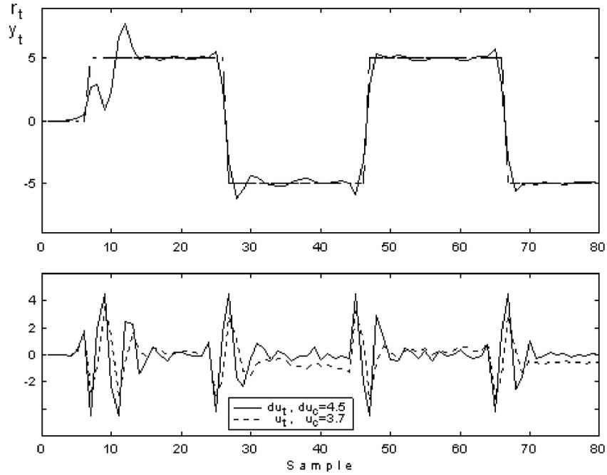
Fig. 13. STGPC under input constraints (Example 1, ARIMAX).
