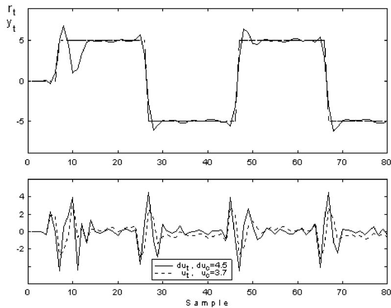
Fig. 12. STGPC under input constraints (Example 1, ARIMAX).
