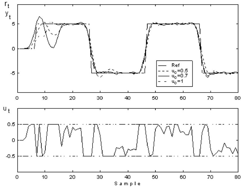
Fig. 7. STGPC under amplitude constraints (Example 1, ARMAX).
