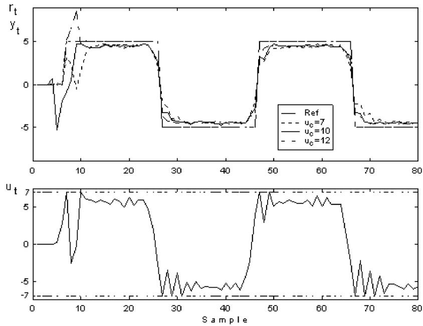
Fig. 8. STGPC under amplitude constraints (Example 2, ARMAX).
