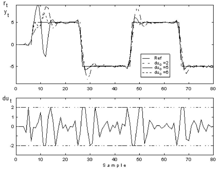
Fig. 1. STGPC under rate constraints (Example 1, ARIMAX).
