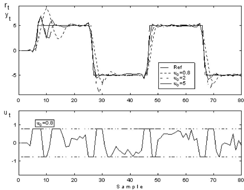
Fig. 6. STGPC under amplitude constraints (Example 1, ARIMAX).
