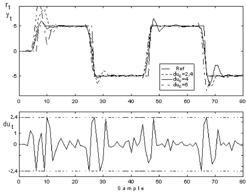
Fig. 2. STGPC under rate constraints (Example 1, ARMAX).
