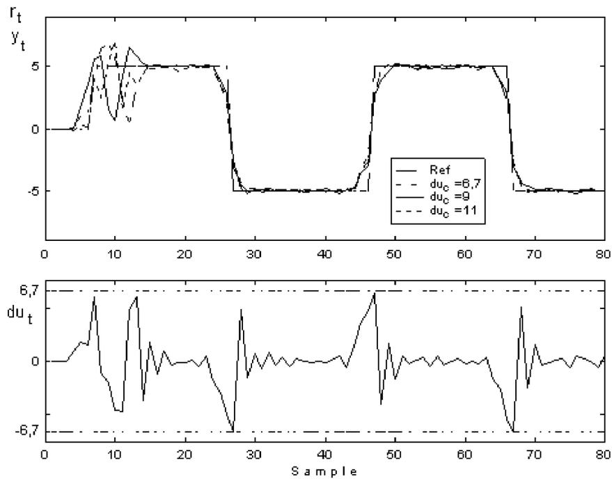
Fig. 4. STGPC under rate constraints (Example 2, ARIMAX).
