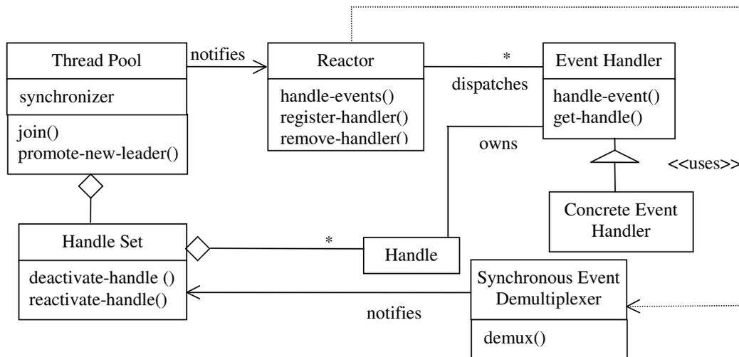
Fig. 4. UML class diagram of the *Reactor-Leader/Followers* pattern combination.
