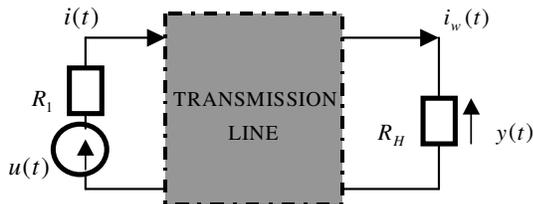
Fig. 1. Scheme of energy transfer.
