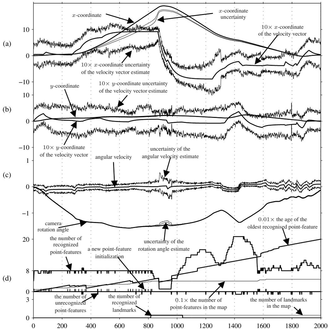
Fig. 8. Runs of real and estimated variables of the SLAM system in the case with a landmark:  $x$ -coordinates (a) and  $y$ -coordinates (b) of the camera position/velocity vector, rotation angle and angular velocity of the camera (c). Estimates are visualized indirectly as trajectory envelopes  $\pm 3\sigma$ . Additional parameters characterising the operation of the system (d).
