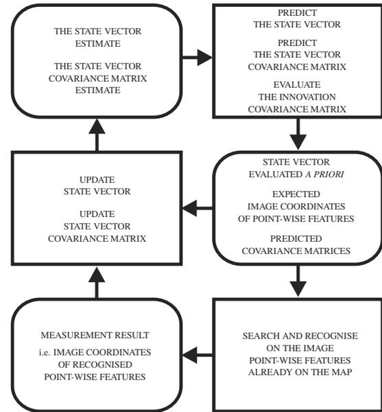
Fig. 1. Cyclic tracking sequence using the EKF scheme in the case of point-wise environment features put on the map.
