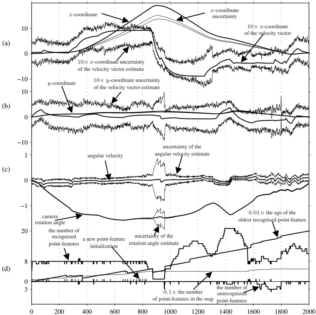
Fig. 6. Runs of real and estimated variables of the SLAM system in the absence of landmarks:  $x$ -coordinates (a) and  $y$ -coordinates (b) of the camera position/velocity vector; rotation angle and angular velocity of the camera (c). Estimates are visualized indirectly as trajectory envelopes  $\pm 3\sigma$ . Additional parameters characterising the operation of the system (d).
