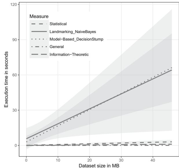
Fig. 3. Meta-feature extraction cost. Only the *Landmarking and Model-Based* class is represented through single measures. The rest of the classes are represented as the total execution times of their participating measures (see Table 2).
