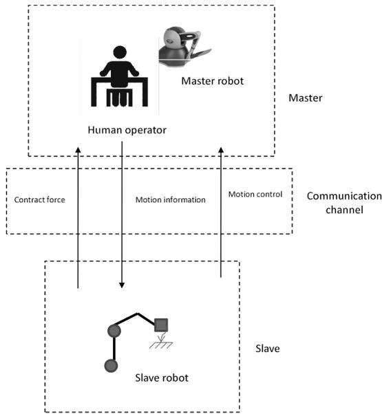
Fig. 2. Bilateral teleoperation with haptic feedback.
