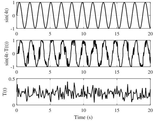
Fig. 3. Delayed signal with a variable time delay.
