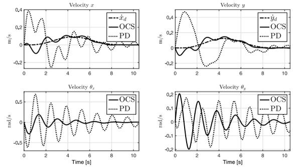
Fig. 3. Comparison of the closed-loop response velocities between OCS and a traditional PD.
