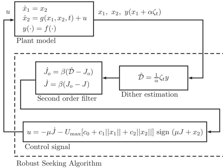
Fig. 1. Block diagram structure for the algorithm.
