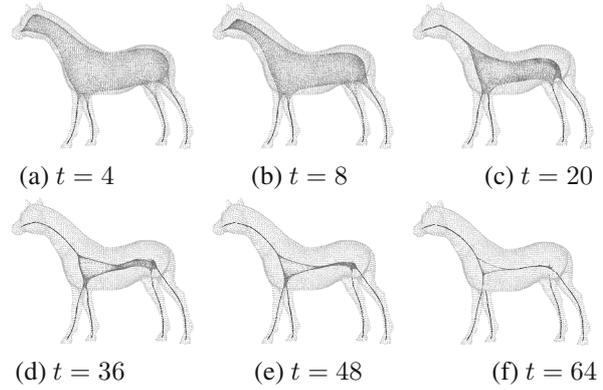
Fig. 3. KNN contraction with gradually increasing  $k$  on the horse model: points belonging to the horse's limbs firstly complete the contraction (a)–(b), as the number  $t$  of iterations increases, points belonging to the larger branches of horse models are contracted to a skeletal structure (c)–(f).
