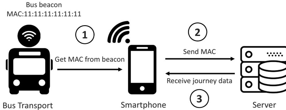
Fig. 2. Proposed outdoor location system schema.
