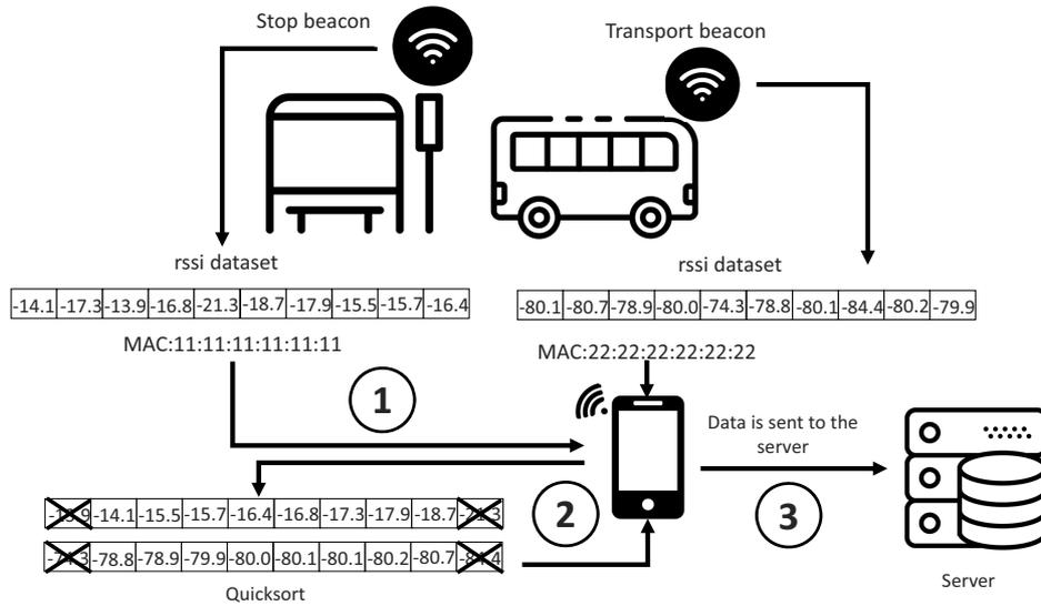
Fig. 3. Proposed beacon-based event detection system.
