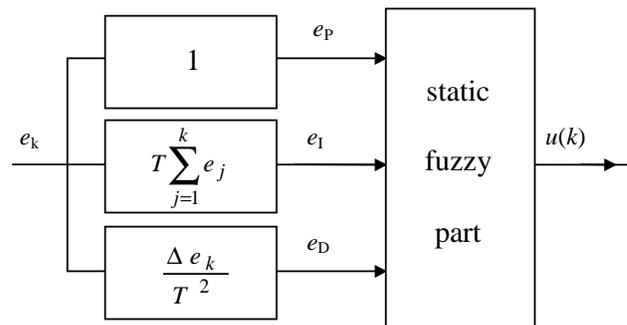
Fig. 2. Inner structure of the fuzzy PID controller.
