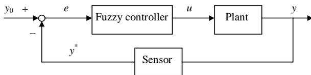
Fig. 1. General scheme of the fuzzy control system.
