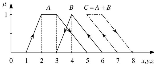
Fig. 16. Addition of ordered fuzzy numbers with opposite orientation according to the method of (Kosiński *et al.*, 2003).
