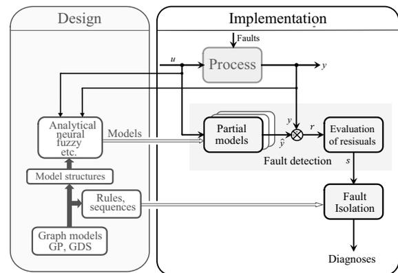
Fig. 3. Scheme of diagnosing with the FDPS approach.
