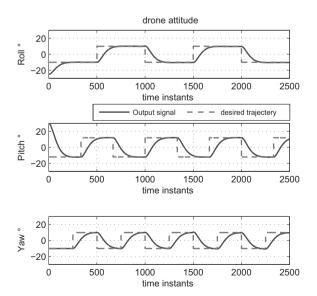
Fig. 3. Quadrotor attitude  $(\varphi, \theta, \psi)$  and reference.
