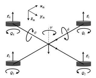
Fig. 2. Quadrator mini-helicopter configuration: the inertial frame  $N(e_{x_n}, e_{y_n}, e_{z_n})$  and the body frame  $B(e_{x_h}, e_{y_h}, e_{z_h})$ .
