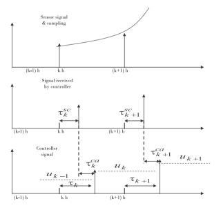
Fig. 5. Timing diagram for data communication.
