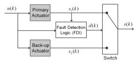
Fig. 1. Duplex actuator system.
