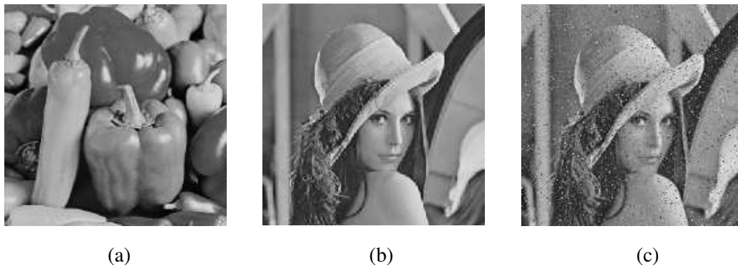
Fig. 2. Test images: (a) original image Peppers , (b) original image Lena , (c) Lena degraded by 10% impulsive noise ( p_v = 0.1 ).
