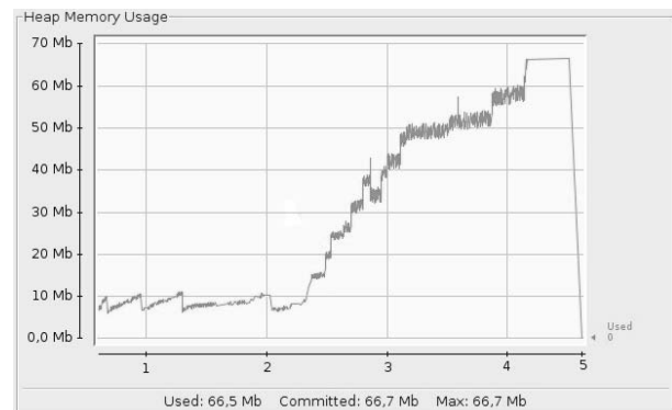
Fig. 8. Increase of memory utilization because of the switch from Ed to Rdv .
