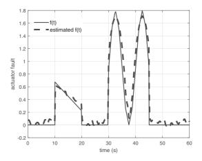
Fig. 2. Actuator fault f(t) and its estimate  $\hat{f}(t)$ .
