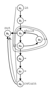
Fig. 7. Complete path in the control flow graph of the function Search.
