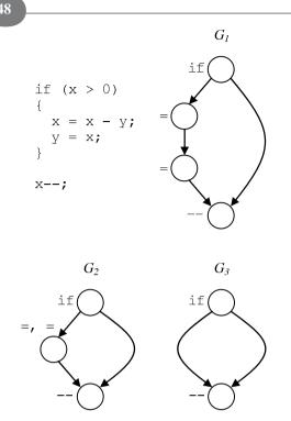
Fig. 14. Example with empty branch and its control flow graph  $(G_1)$ , segment graph  $(G_2)$  and program graph reduced to segments (Paige, 1977) as a graph with multiple edges  $(G_3)$ .
