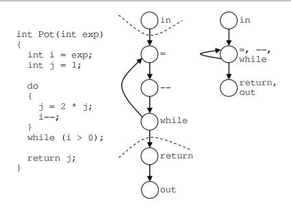
Fig. 6. Function Pot, control flow graph and segment graph.
