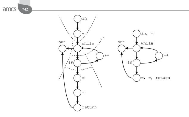
Fig. 5. Control flow graph and segment graph of function Search.
