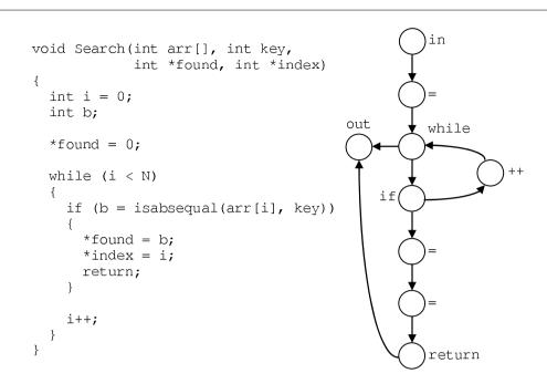
Fig. 1. Function Search and its control flow graph.
