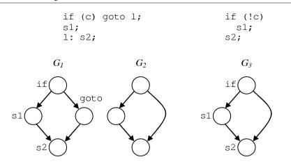
Fig. 12. Example with goto and its segment graph  $(G_1)$  and program graph (Rapps and Weyuker, 1982)  $(G_2)$ ; the same example without goto and its segment graph  $(G_3)$ .
