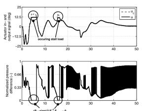
Fig. 5. Stall loads during a high input maneuver.
