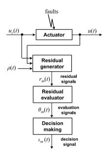
Fig. 1. FDD system for parametric LOE monitoring.
