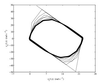
Fig. 3. Stick-slip limit cycle.
