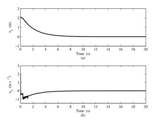
Fig. 6. Axial trajectories of the closed loop system (6), (28)–(29):  $x_1 = Y - \Gamma_0 t$  (a),  $x_2 = \dot{Y} - \Gamma_0$  (b). Variables Y and  $\dot{Y}$  represent the axial position and axial velocity, respectively.
