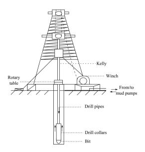
Fig. 1. Basic scheme of a vertical drilling system.
