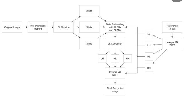
Fig. 4. Block diagram of reference image encryption of Scheme 2.
