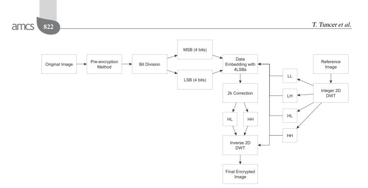
Fig. 3. Block diagram of reference image encryption of Scheme 1.
