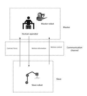
Fig. 2. Bilateral teleoperation with haptic feedback.
