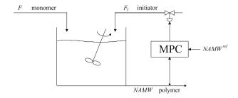
Fig. 4. Polymerisation reactor control system structure.
