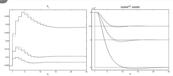
Fig. 8. Simulation results of the polymerisation reactor with the MPC-NPL (dashed line) and MPC-NO (solid line) algorithms with the neural network model: the set-point point changes from NAMW = 40000.
