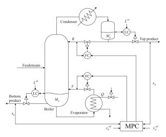
Fig. 9. Distillation column control system structure.
