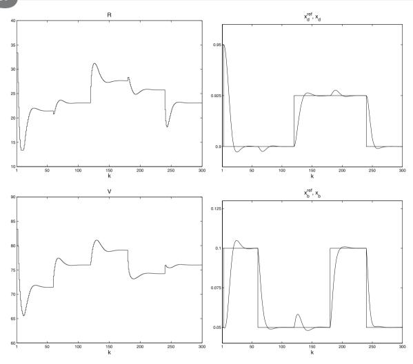
Fig. 10. Simulation results of the distillation column with the MPC algorithm with the linear model
