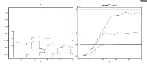
Fig. 5. Simulation results of the polymerisation reactor and the MPC algorithm and the linear model valid for a low NAMW level: the set-point point changes from NAMW = 20000.
