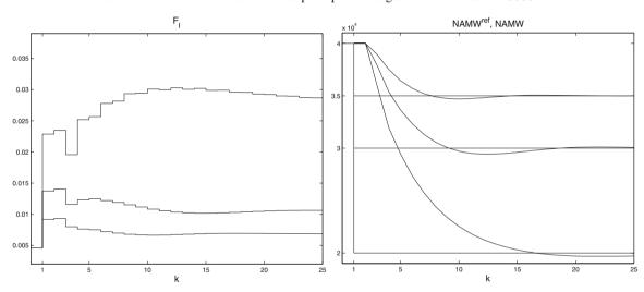
Fig. 6. Simulation results of the polymerisation reactor with the MPC algorithm with the linear model valid for a high NAMW level: the set-point point changes from NAMW = 40000.
