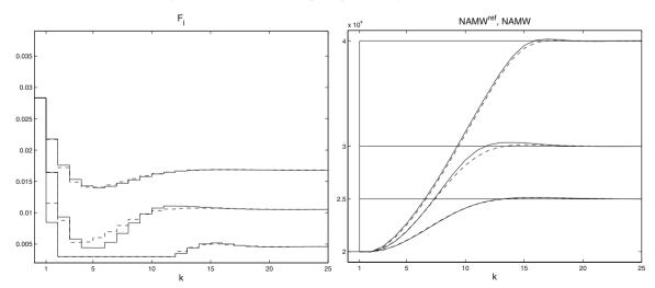
Fig. 7. Simulation results of the polymerisation reactor with the MPC-NPL (dashed line) and MPC-NO (solid line) algorithms with the neural network model: the set-point point changes from NAMW=20000.
