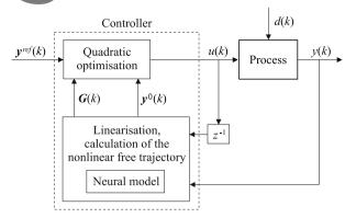
Fig. 3. Structure of the MPC algorithm with Nonlinear Prediction and Linearisation (MPC-NPL). Here d(k) constitutes the unmeasured disturbance.
