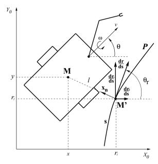
Fig. 5. Illustration of the path following problem for a nonholonomic platform.
